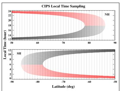
**Figure 1**. Local time sampling of the CIPS level 2 measurement pixels for a typical orbit in the Northern Hemisphere (top panel) and Southern Hemisphere (bottom panel). Black and red points denote the descending and ascending portions of the orbit, respectively. Vertical lines represent boundaries of the latitude bins used in the Level 3c summary files.
