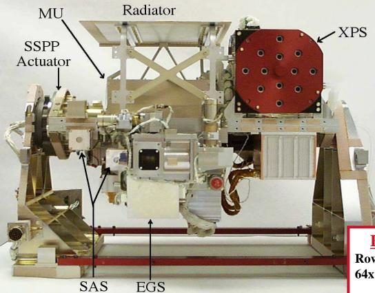
MU = Microprocessor Unit SSPP = SEE Solar Pointing Platform SAS = Solar Aspect Sensor (2) Measures the solar vacuum ultraviolet (VUV) irradiance Range: 0.1-194 nm Resolution: 0.4 nm EGS (27-194 nm) 5-10 nm XPS (0.1-34 nm) Measurement Cadence: 10-sec integrations, but only for 3 min per orbit (96 min)
