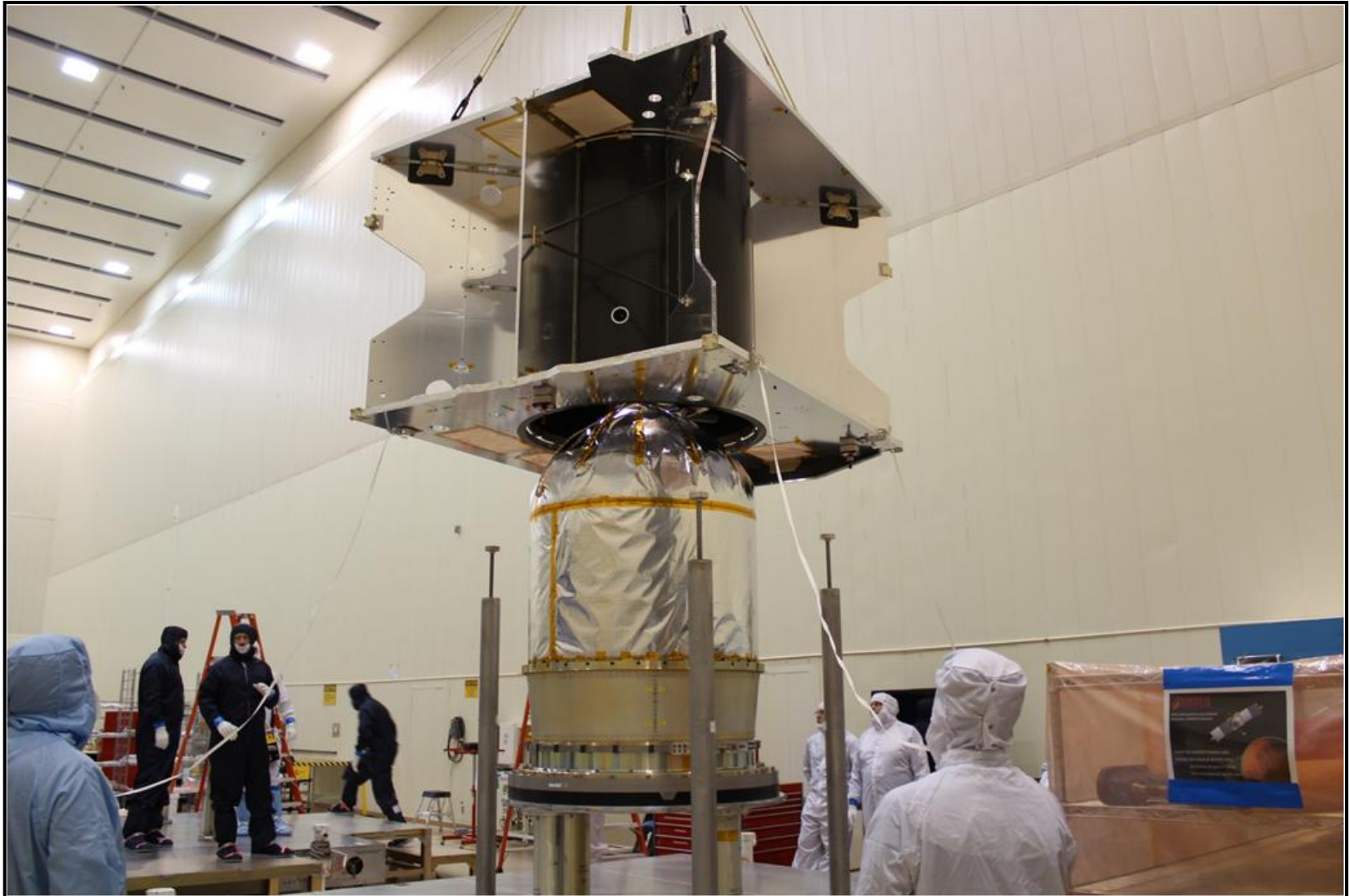
Integration of core structure with fuel tank
