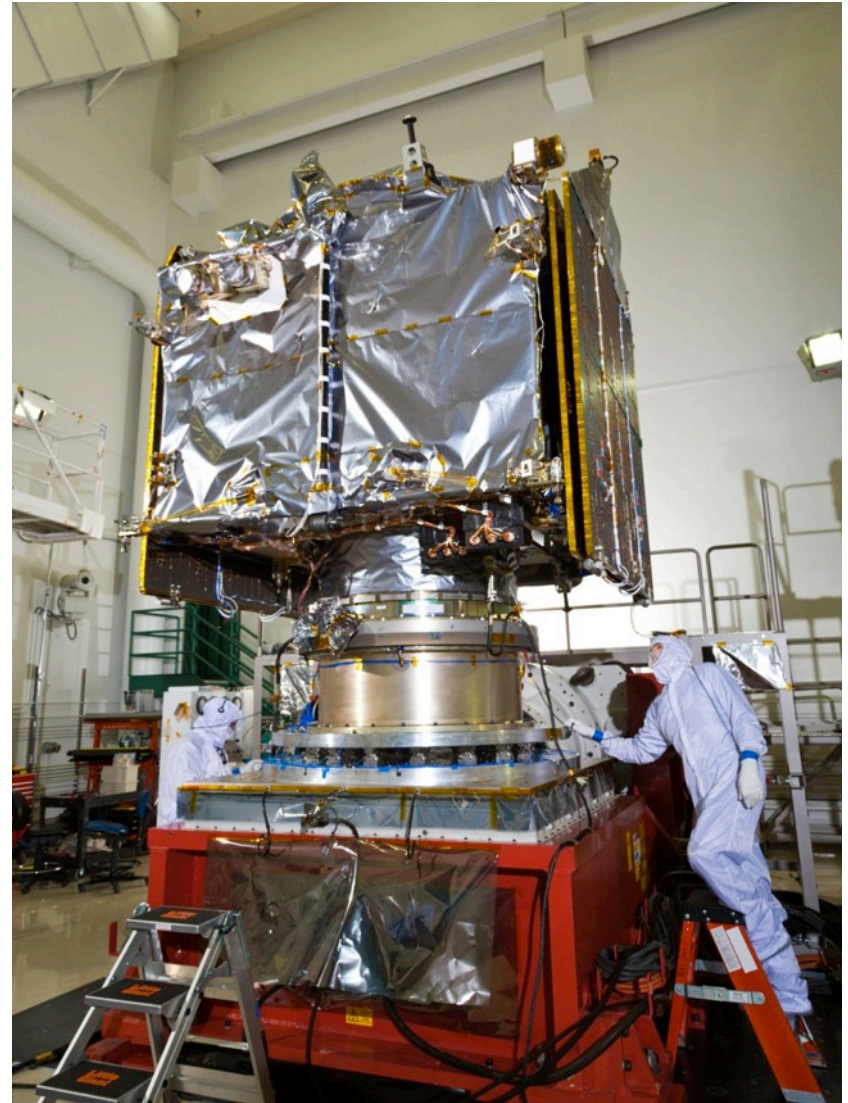
MAVEN on Shaker – Sine Vibration
