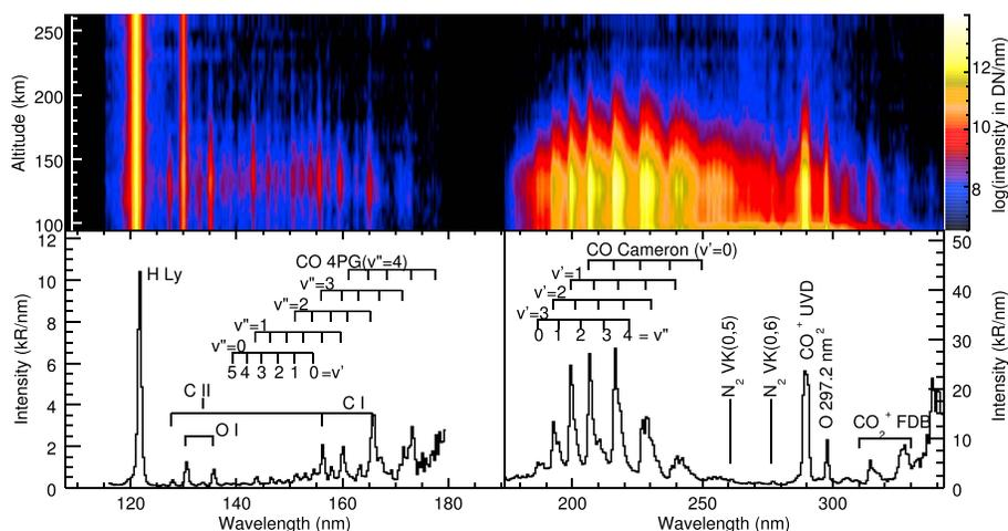
**Figure 1.** (top) The IUVS’s FUV and MUV detectors color composite generated using a full vertical scan from orbit 110 (2059 UTC, 18 October 2014), one of the 744 profiles. The horizontal and vertical axes represent wavelength and altitude (80–250 km), respectively. (bottom) Calibrated FUV and MUV spectra obtained from the same scan; these are averages of 13 individual spectra obtained between 120 and 135 km.
