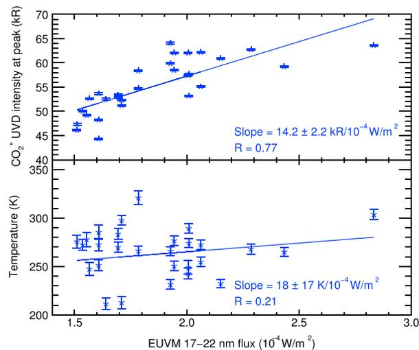
**Figure 5.** Short-term variations of (top)  $\text{CO}_2^+$  doublet maximum intensity and (bottom) topside temperature with 17–22 nm irradiance measured by the EUVM instrument aboard MAVEN. Values are for  $L_S \sim 337\text{--}343^\circ$  (orbits 1160–1220) and SZA between  $30^\circ$  and  $40^\circ$ .  $R$  is the linear correlation coefficient.
