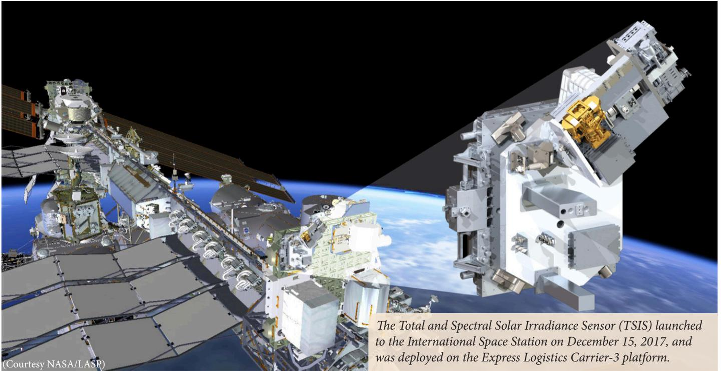
The Total and Spectral Solar Irradiance Sensor (TSIS) launched to the International Space Station on December 15, 2017, and was deployed on the Express Logistics Carrier-3 platform.
