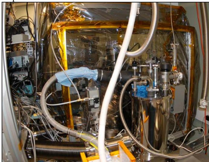
A NIST-calibrated cryogenic radiometer (foreground) accurately measures input light at solar power levels in the TRF. Instruments are tested in the vacuum chamber enclosed by the clean tent toward the rear.
