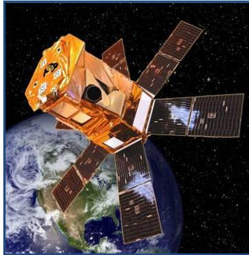
2008) and is currently in the sixth year of its extended mission. It has achieved its primary mission goal of measuring total solar irradiance (TSI) and solar spectral irradiance (SSI) in the 0.1-27 nm and 115-2400 nm wavelength ranges with unprecedented accuracy and precision. The main objectives of the *SORCE* extended mission are very much aligned with the original *SORCE* mission objectives, but have new focus with the current state of NASA missions and solar activity in solar cycle 24.
