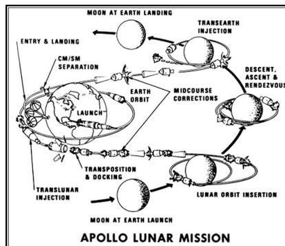
The Apollo 11 spacecraft was launched from Cape Kennedy at 13:31:01 GMT on July 16, 1969. After 2 hr and 33 min in Earth orbit, the S-IVB rocket engine was reignited for acceleration of the spacecraft to the velocity required to escape Earth's gravity. Although at times the spacecraft reached speeds near 40,000 km/hr, the average speed was about 5500 km/hr .
