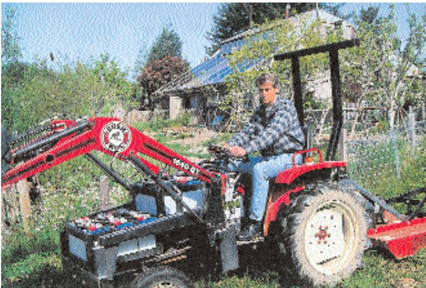
Renewable-energy specialist Stephen Heckerroth driving his electric tractor. He uses solar panels (including those visible on the barn roof in the background) to charge the batteries that power the tractor.
