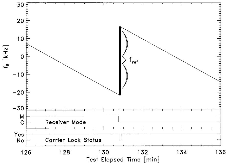
Figure 9. Upper panel: Measured frequency  $f_R$  during a 10 min interval about the switch from mission to checkout mode; Middle panel: Receiver Mode ('C' = checkout; 'M' = mission); Lower panel: Carrier Lock Status. The best fit value for  $f_{ref} = 38\,504.2$  Hz was obtained from the vertical displacement of the two lines.
