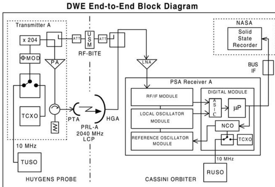
Figure 6. DWE experiment configuration (reprinted from Bird *et al.*, 1997b).
