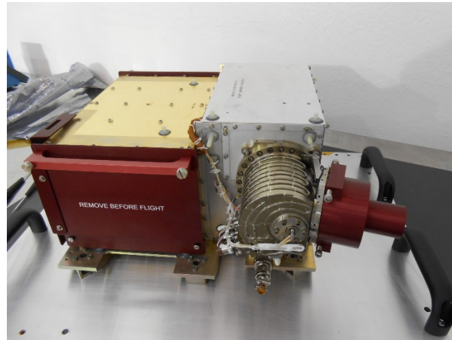
Figure 1: The MAVEN NGIMS Instrument during Integration and Testing (I&T).
