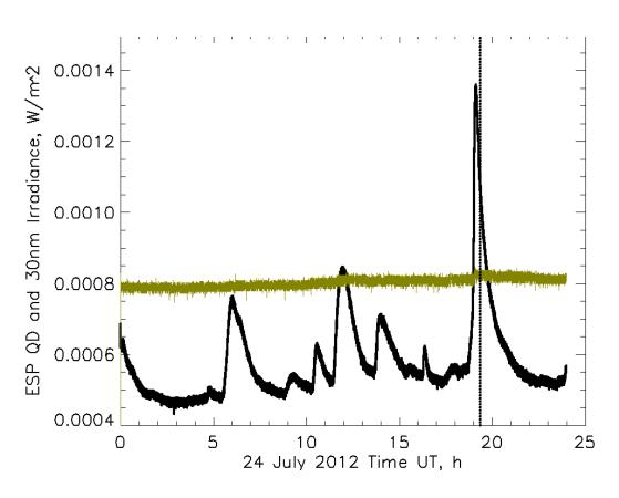
ESP Ch9 (27.16 – 33.8 nm) irradiance for the 36.263 flight apogee time (dotted line) is **8.2E-4 W/m^2**.
