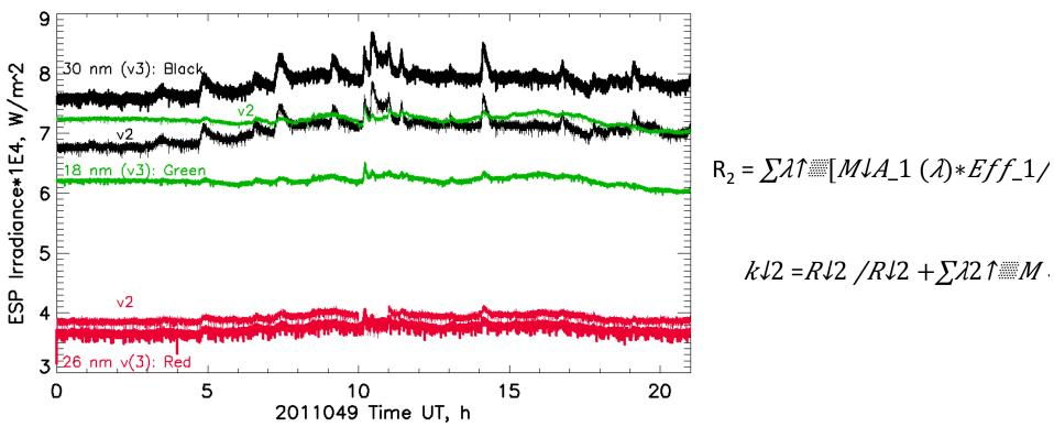
v3 (thick) vs v2 (thin) difference is related to **a)** corrected MA and MB tables, **b)** updated bandpass edges, and **c)** updated  $2^{nd}$  order coefficients ( $k_2$ ) as a result of EVE SR flight
