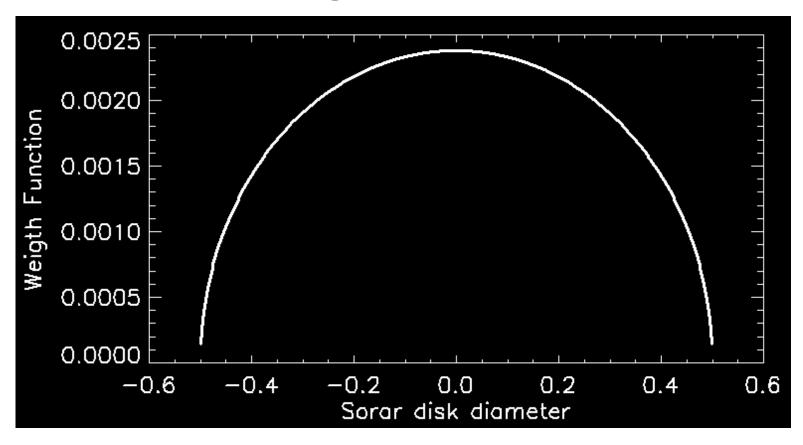
The whole disc area (-0.267 to +0.267 deg) was divided on 535 slices ( $\Delta \alpha$  =0.001 deg) along the dispersion direction. Weight of each slice (W) and interpolated efficiency (Eff) were determined.
