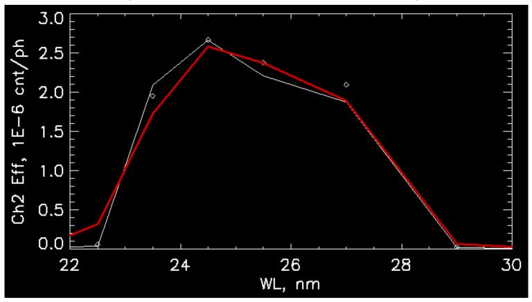
Calculated profiles (red) are compared to the original ESP flight efficiency profiles (thin white line) previously used as inputs for convolution with the slit function. Diamonds are based on TW suggestion to use three area model (central with the weight of 0.94 and two edge areas with the weight 0.03 each).
