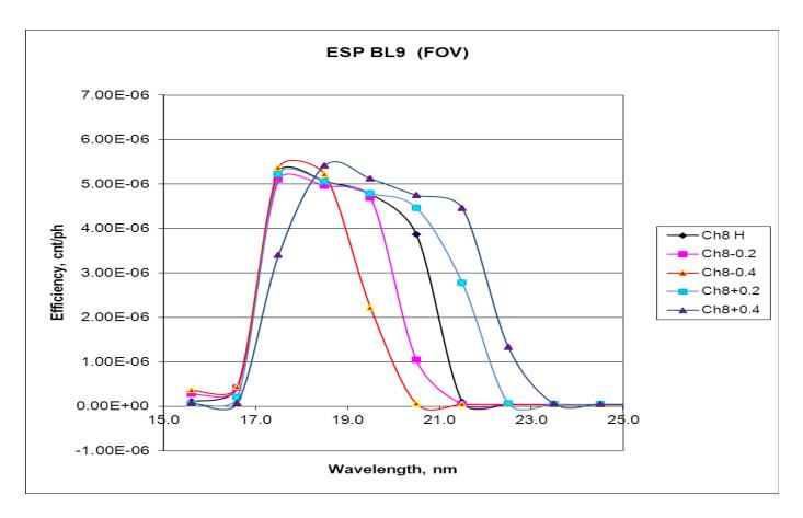
The edges (Dec 2011 – Jan 2012) were determined using SURF BL-9 Flight efficiency profiles (Ch8 shown) for both centered and tilted (± 0.4 and (± 0.2 deg) ESP positions.
