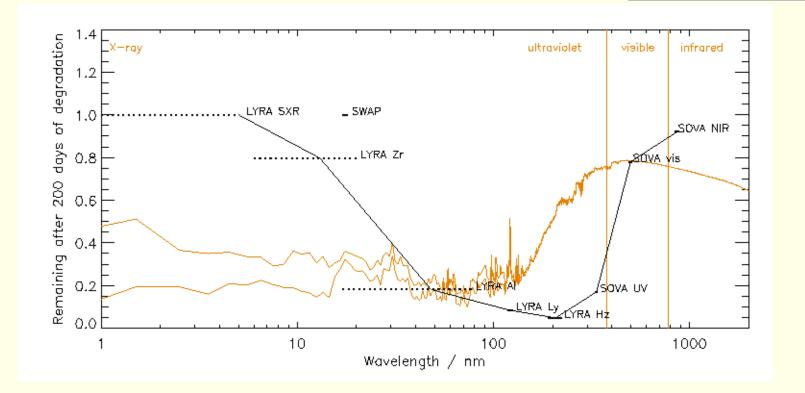
EURECA / SOVA1992-1993 (retrieved by Space Shuttle)PROBA2 / LYRA2010-2012UV-polymerization -> molecular contamination on first optical surface
