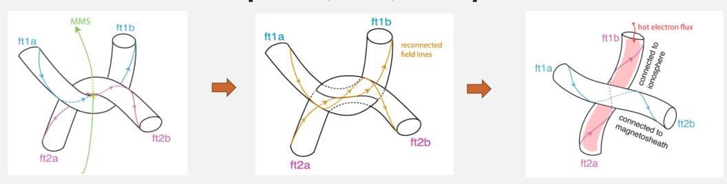
This may explain the equal occurrence of flux ropes (a) filled with (b) devoid of hot electrons [Russell & Qi, 2019]
