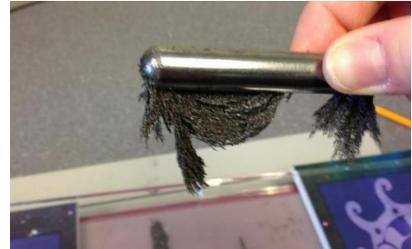
Figure 4. Iron filings attracted to cow magnet.
