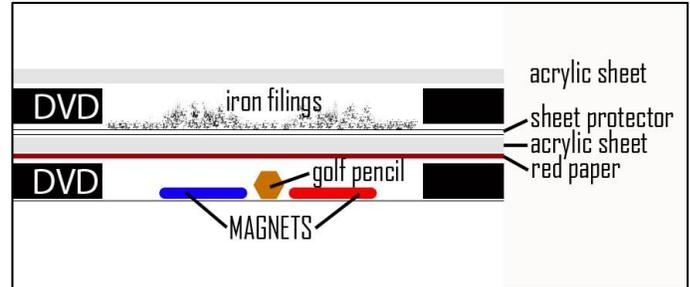
Figure 7. Profile diagram of a completed model after step 15.
