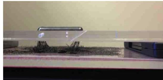
Figure 8. Iron filings attracted to the cow magnet and jumping up to the underside of the acrylic sheet.
