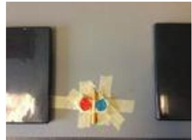
Figure 5. Two DVD cases flanking the taped down magnets.
