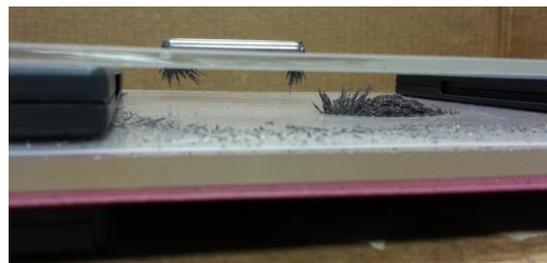
Figure 9. Cow magnet pulling away iron filings from the underlying magnets.
