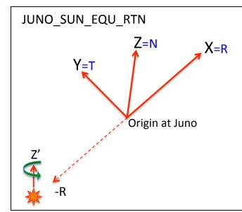
Figure 6 – This system is centered with *Juno* at the origin and the relative object is the Sun.
