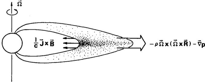
Fig. 1. Force balance in a rotating plasma. The outward centrifugal and pressure gradient forces are balanced by an inward Lorentz force.
