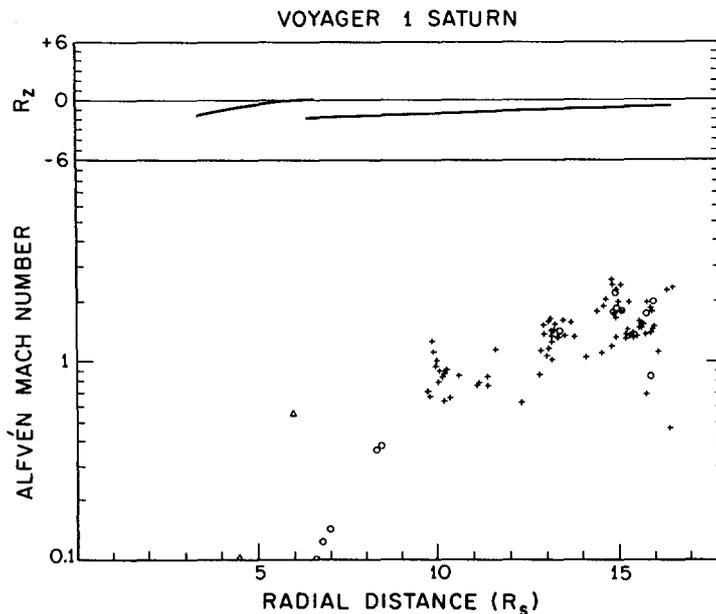
Fig. 3 The bottom panel shows Alfvén Mach numbers derived from MAG and PLS data (O inbound high resolution, + inbound low resolution,  $\Delta$  outbound high resolution PLS spectra). The top panel shows vertical distance from the MEP. Both panels are plotted versus radial distance.
