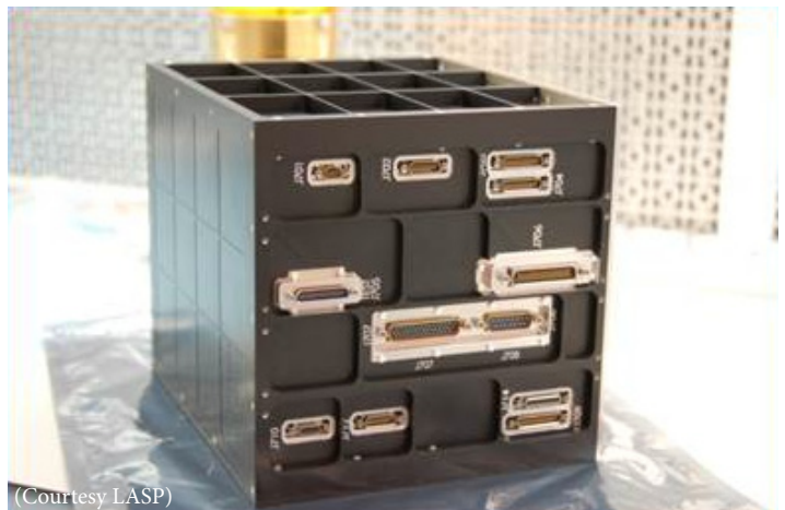
SORCE Microprocessor Unit in mother/daughterboards configuration
