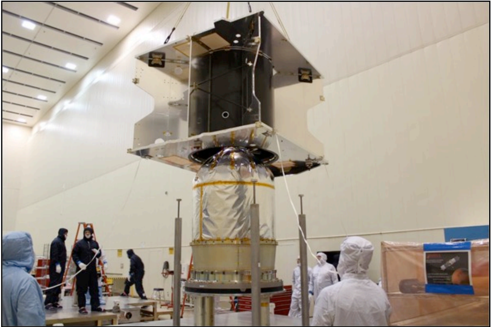
Integration of core structure with fuel tank
