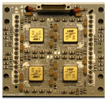
**GOES EUVS-AB Detector Board**—Four custom 6-channel ASICs on a 2" x 2" board provide femtoamp electrometers with 20-bit ADC measurements for the GOES-R EXIS extreme ultraviolet spectrometer in a custom, qualified 52-pin CQFP.
