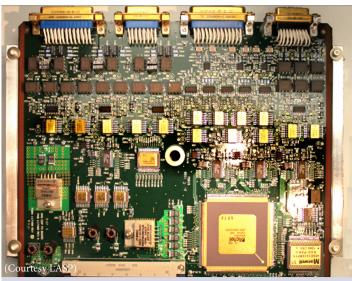
MMS Fields DSP Board—18 Bessel filter channels sampled at up to 250kSps feed the FPGA performing nine simultaneous 1024 point FFTs at 16kHz along with other DSP operations.
