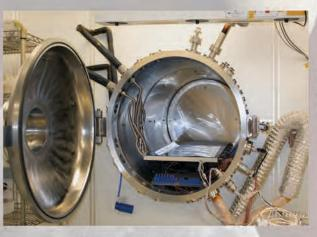
Bemco East •Cryo-Torr 8 HV pump •Ion gauge with high voltage interlock •SRS RGA 200 •Can be set up with QCM Research
