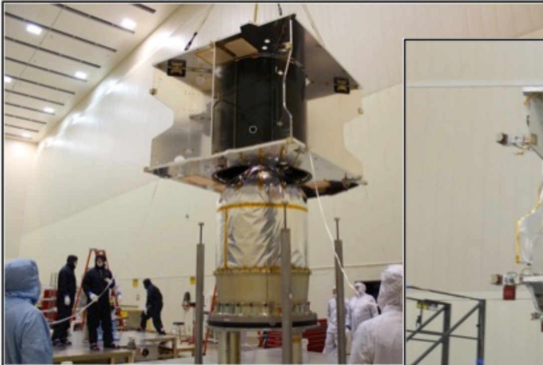
Integration of core structure with fuel tank
