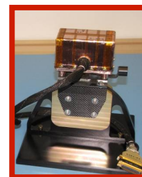
Langmuir Probe and Waves; Bob Ergun, LASP
