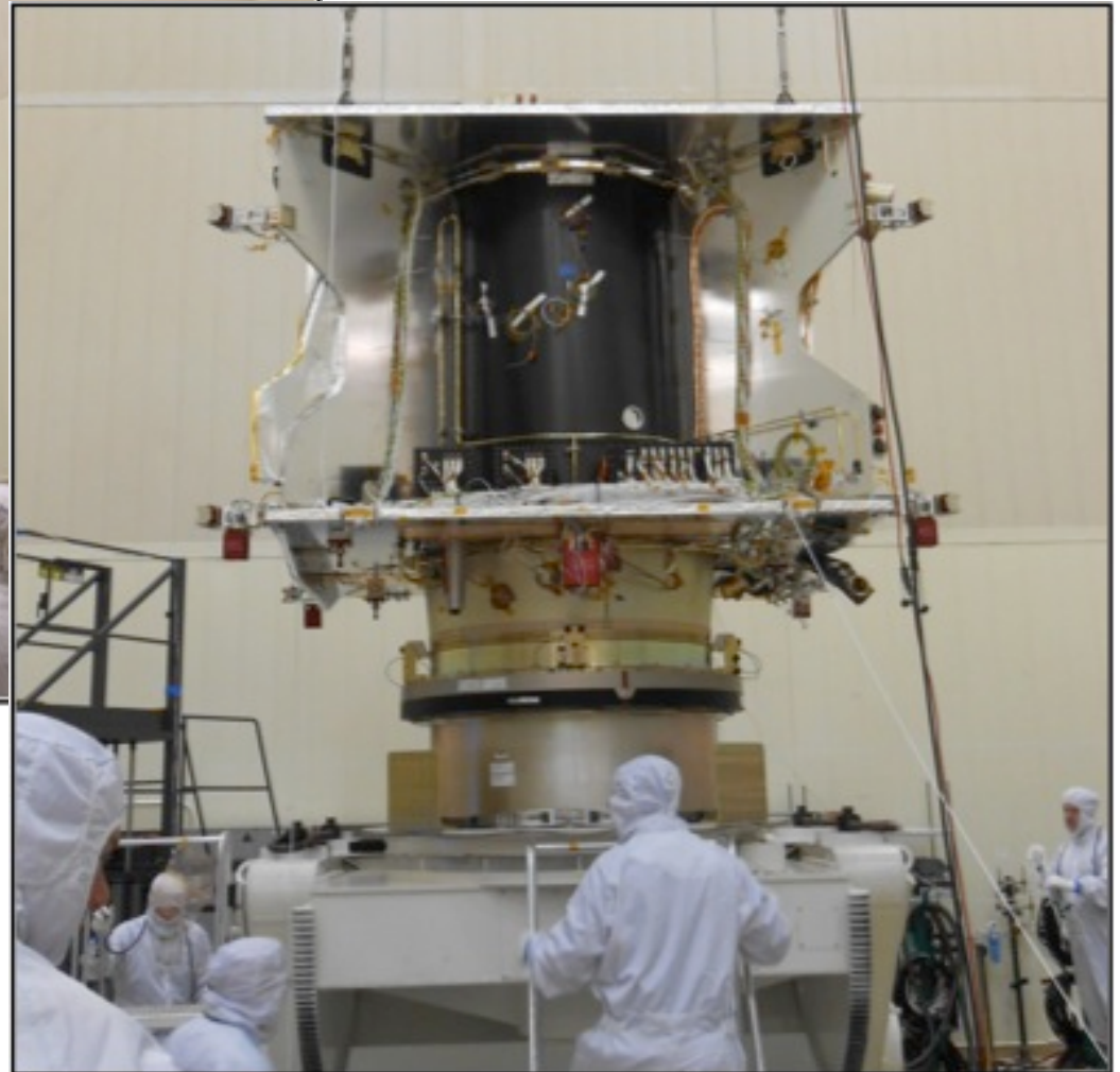
Lift onto rotation fixture, for easier access
