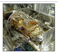
TSIS SIM in the LASP Spectral Radiometry Facility (SRF) Vacuum Tank.
