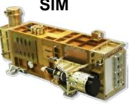
Solar spectral irradiance is solar energy as a function of wavelength, needed to understand how the Earth system responds to changes in irradiance. The TSIS SIM is a 3-channel prism spectrometer to measure full-disk SSI at 200 -2400 nm wavelengths.
