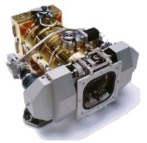
**Total solar irradiance** is the dominant energy source driving the Earth's climate system. The TSIS TIM contains four ESRs to provide full-disk TSI measurements with the capability to track degradation. It will continue a 40-year uninterrupted measurement record of TSI.
