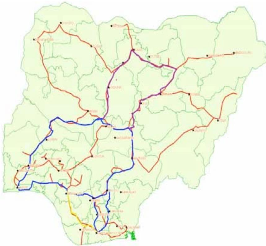
Figure 6. MTN Nigeria's national microwave and fibre optics transmission network. . Red = SDH Microwave; blue = MPLS Fibre rings 1&2; purple = MPLS Fibre Ring 3; yellow = MPLS Fibre Ring 4 Source: Chukwuma et al. (2009), courtesy of MTN Nigeria
