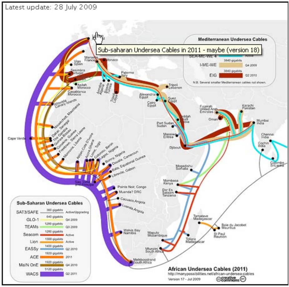
Figure 4. Submarine cable projects for Africa to be completed by 2011. The map is kept current by Steve Song and is available on the Internet together with details on the completion dates, ownership, capacity etc.
