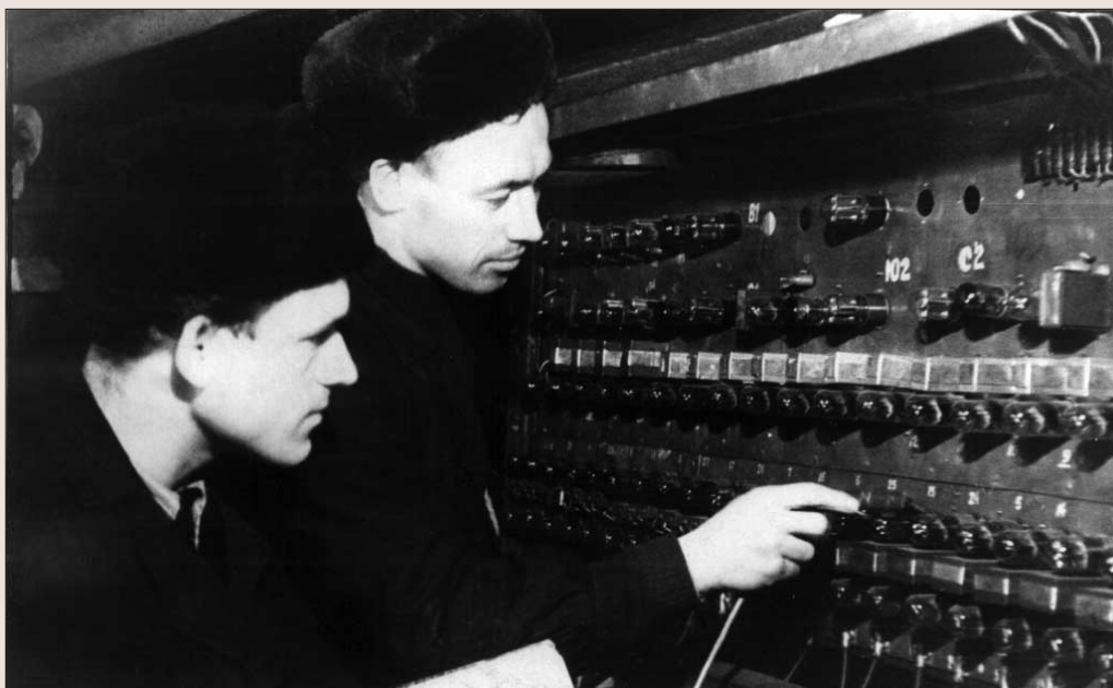
Figure 2. Photo from 1956 taken at the Yakutsk Branch of the USSR Academy of Sciences. Radio technicians S. N. Druzhinin and V. P. Razin undertake the calibration of muon counters in a shaft at a depth of 60 m. The extensive underground research complex at Yakutsk provided data for many important research papers and doctoral dissertations. (Photo provided by Sergei Druzhinin and Sergey Starodubtsev).
