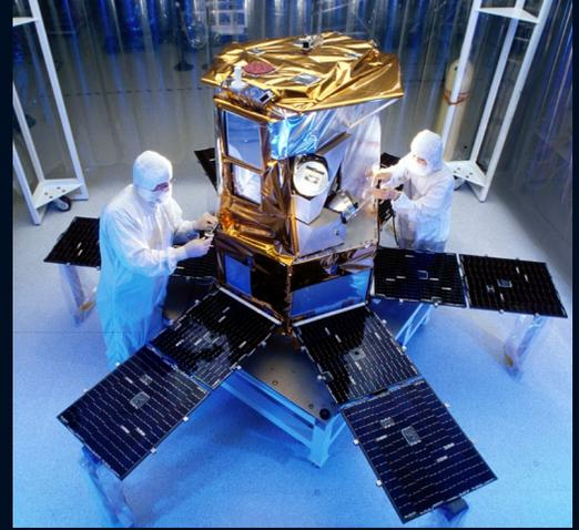
TSIS-1 is 363 kg built by LASP mounted to the ISS
