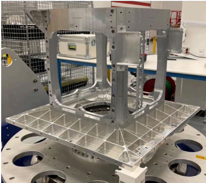
Flight PIU module in burn in chamber
