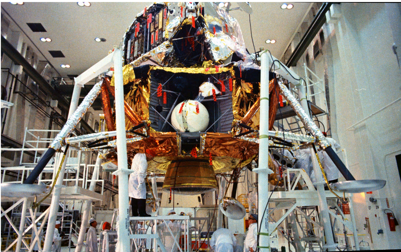
Final systems checkout for NASA's Lunar Module (LM-5) are conducted in the Open Bay Area of the Manned Spacecraft Operations Building.
