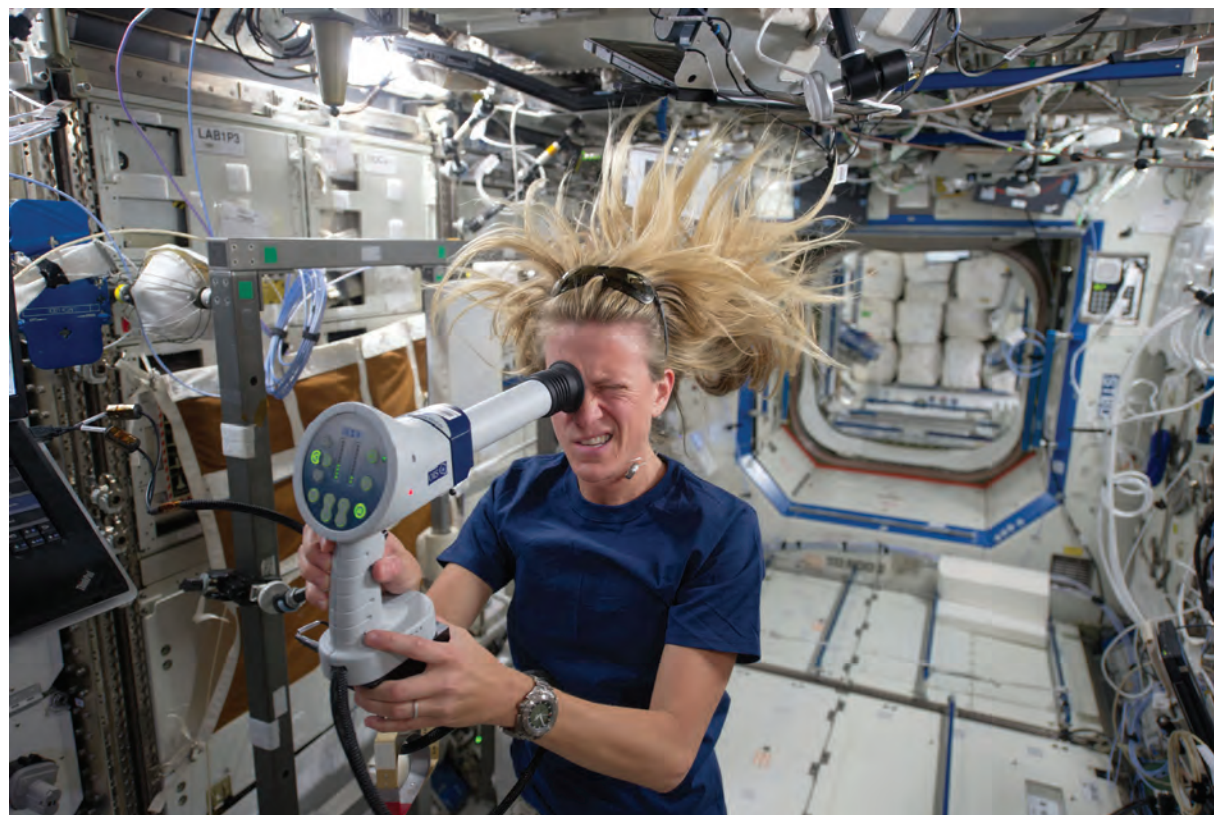
FIGURE 2.3 Expedition 36/37 Flight Engineer Karen Nyberg of NASA uses a fundoscope to take still and video images of her eye while in orbit. This was the first use of the hardware and new vision-testing software. SOURCE: Courtesy of NASA, http://www.nasa.gov/content/it-s-all-in-your-head-nasa-investigates-techniques-for-measuring-intracranial-pressure/ .
