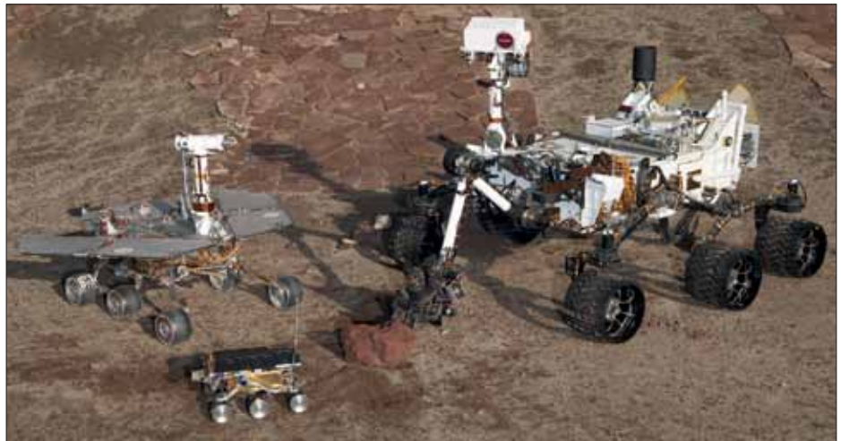
1: The increasing size of Mars rovers, from Pathfinder (front left), a Mars Exploration Rover (left), to Mars Science Laboratory (right). This increase in size (and cost), contrary to predictions that improved technology will result in smaller and cheaper robots, is mandated by the nature of the martian surface and complexity of exploration objectives. Human missions would be even larger and more expensive, but, crucially, much more capable. (NASA/JPL-Caltech)
