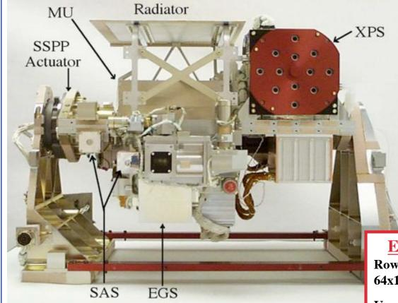
MU = Microprocessor Unit SSPP = SEE Solar Pointing Platform SAS = Solar Aspect Sensor (2) Measures the solar vacuum ultraviolet (VUV) irradiance Range: 0.1-194 nm Resolution: 0.4 nm EGS (27-194 nm) 5-10 nm XPS (0.1-34 nm) Frequency: 10-sec integrations, but only for 3 min per orbit (96 min)
