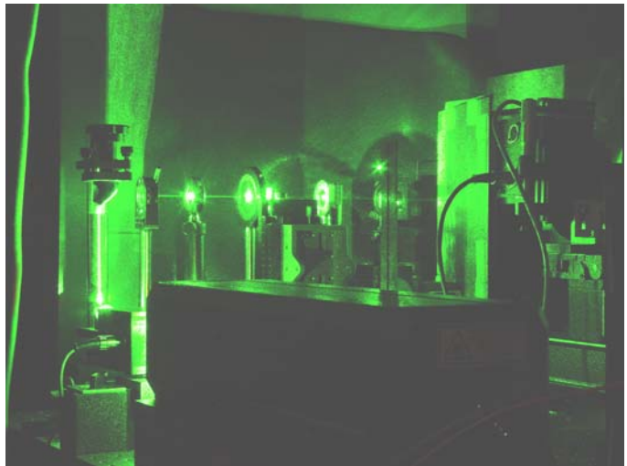
Figure 2. The NIST laser and optics provide a stable, high-power illumination source for the TIM.
