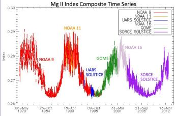
Magnesium II Core-to-Wing Index Composite Time Series. This proxy for solar activity has been continuously measured since 1978 by a variety of instruments operated by both NOAA and NASA. SORCE SOLSTICE has been making daily measurements since its launch in 2003.
