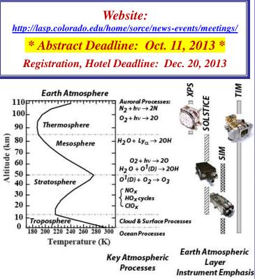
This figure represents a synopsis of the primary studies with SORCE data. The SORCE total and spectral radiometers measure daily the spectrum of the Sun and its variability. Solar energy establishes the structure of Earth's atmosphere through a series of key chemical reactions and thermodynamic processes. The SORCE instruments were designed to provide input for studying different layers of Earth's atmosphere and influences on climate change.
