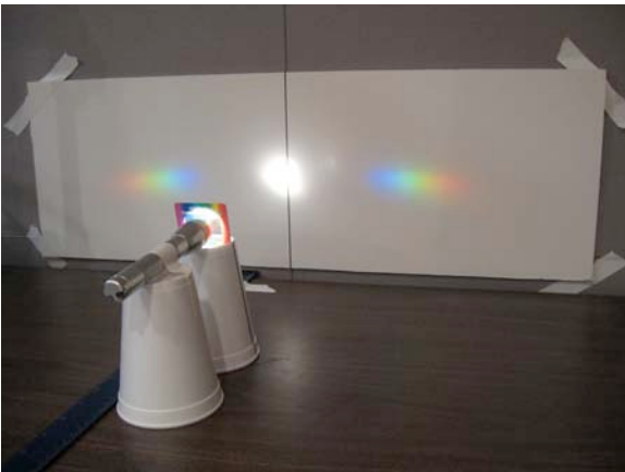
Image 7: Place the flashlight stand directly behind the grating stand to form a spectrum on the screen.
