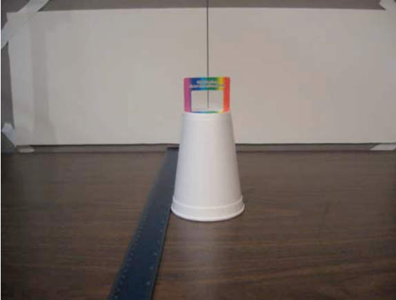
Image 6: The set-up is almost complete. Place the grating stand in front of the screen. The meter stick is perpendicular to the screen and also touching the side of the grating stand.
